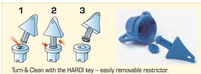
Turn-&-Clean with the HARDI key – easily removable restrictor.
